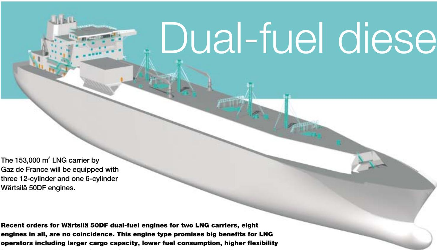
The 153,000 m<sup>3</sup> LNG carrier by Gaz de France will be equipped with three 12-cylinder and one 6-cylinder Wärtsilä 50DF engines.
