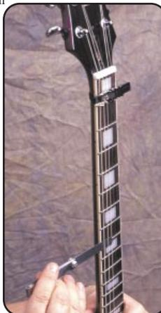
truss-rod nut clockwise. Too convex—Counter clockwise. Check your tuning, then check the gap again with the feeler gauge. In either case, if you meet excessive resistance or need for adjustment, or you're not comfortable with this adjustment, take your guitar to your authorized Service Center.
