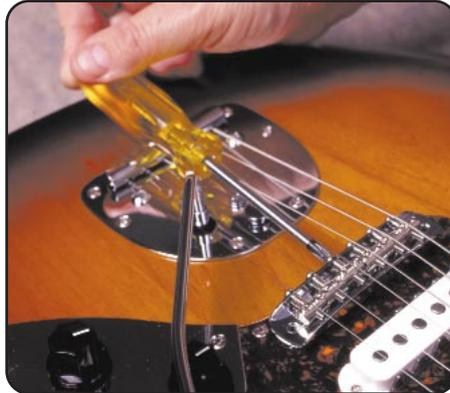
2nd string as a measurement (Example: If the 2nd string is .011" you would move the 2nd string back .011" from the 1st saddle). Move the 3rd back from the 2nd saddle, using the gauge of the 3rd string as a measurement. The 4th string saddle should be set parallel with the 2nd string saddle. Proceed with the 5th and 6th in the same method used for strings 2, and 3.
