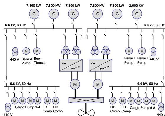
**Figure 4: STX Shipbuilding electric propulsion system diagram**
