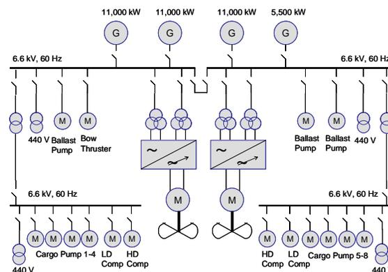
**Figure 3: Twin screw electric propulsion system diagram. Image courtesy of ABB Marine**
