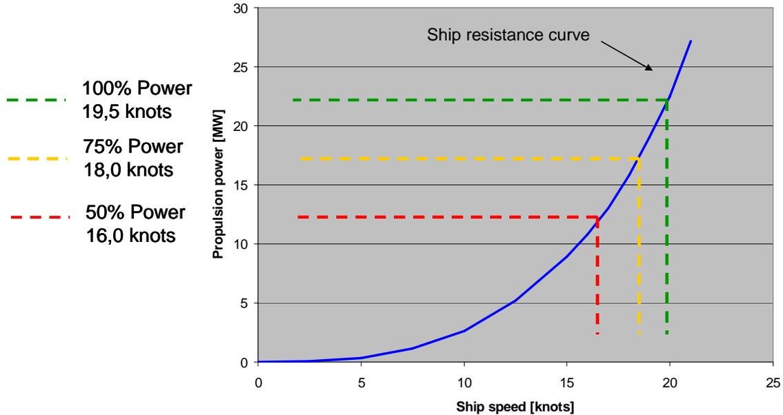
Figure 5: Power - speed curve for an LNGC.
